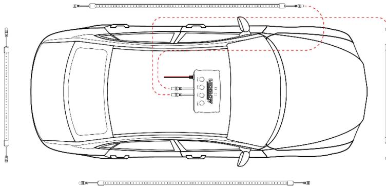
**Note:** There are two male plugs coming out of the control box. Ensure that you have one male plug from the control box plugged into the female end of the driver side tube and the other male plug from the control box plugged into the female end of the front tube. Each underbody tube daisy chains to the next with the included 6 feet of power wire and modular connectors.
