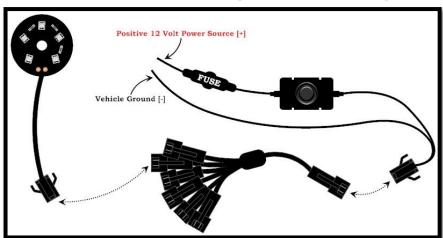
3. Begin by first laying out the pod lights similar to the way they will be installed. Make sure that the wires will be able to be routed in such a way that they will not be pinched, cut or exposed to heat. Also, keep the pod lights and wires away from all moving parts that may come in contact with any part of the kit. IF A POWER WIRE IS PINCHED, IT WILL CAUSE THE KIT TO MALFUNCTION AND WILL VOID THE WARRANTY DUE TO PHYSICAL DAMAGE.
